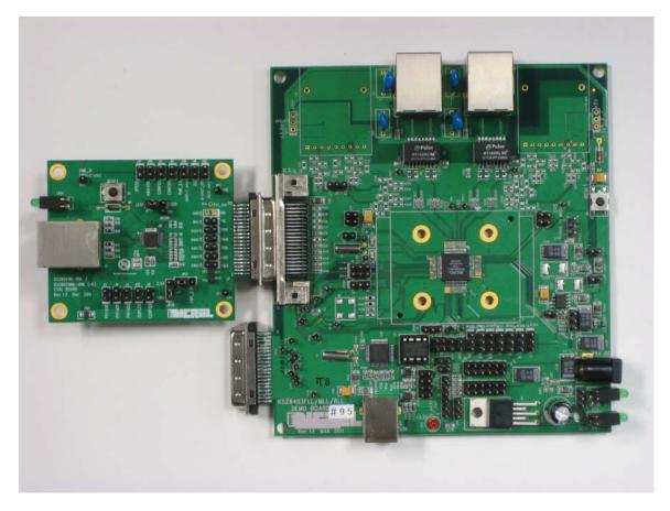
Figure 2. KSZ8081RNB-EVAL interfacing with KSZ8463RLI Evaluation Board
